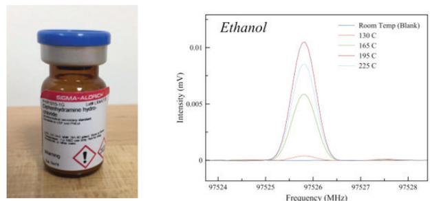
**Figure 2:** Thermal evolution analysis of diphenhydramine hydrochloride (top left). Top right: signal of evolved ethanol in relation to vial temperature. Bottom: broadband spectrum showing a clear match to the FT-MRR signature of ethanol.
