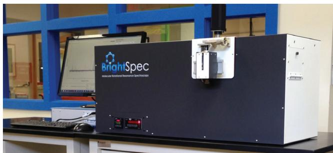
**Fig 1:** BrightSpec One FT-MRR spectrometer with headspace module used for thermal evolution analyses.
